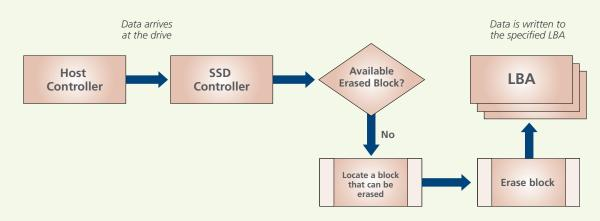
Figure 3: Two-step write process on a full drive—erase, then write. (Additional details are available in the Micron technical marketing brief "Media Management in Solid State Drives: Multistep WRITE Operations.")
